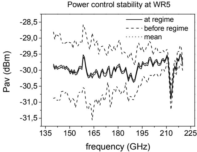
Fig. 6. Stability of the power control in the WR-5 waveguide band. The dashed lines represent the stability boundaries defined using the standard deviation extracted from the 100 measurements considered in Fig.5. The solid lines define the stability boundaries using the standard deviation extracted from measurements when thermal stability is reached.
