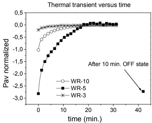
Fig. 5. Average available power, normalized to the regime value, measured at port-1 of the designed setup, for WR-10, WR5 and WR-3 waveguide bands, for the same power set from the user equal to -30 dBm, over 100 consecutive measurements.
