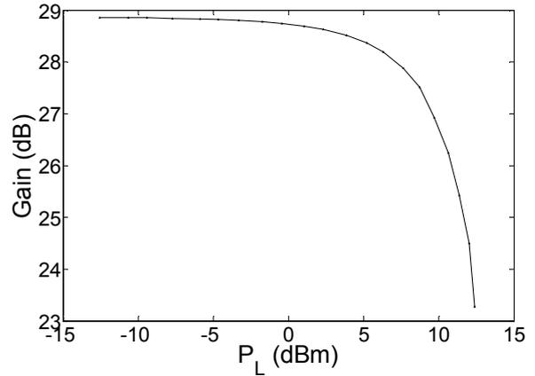
Fig. 7. Gain vs. power delivered to the load measured for a Norden Millimeter N09-2412 amplifier at 90 GHz
