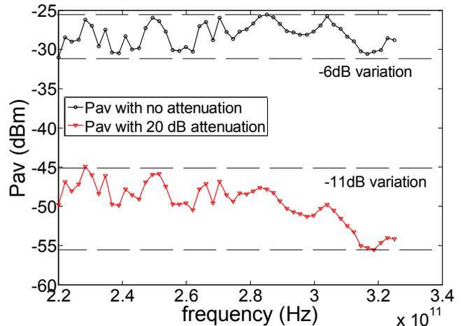
Fig. 1. Output power versus frequency of a mm-wave extender module in the WR-03 range, at different value of external attenuation.
