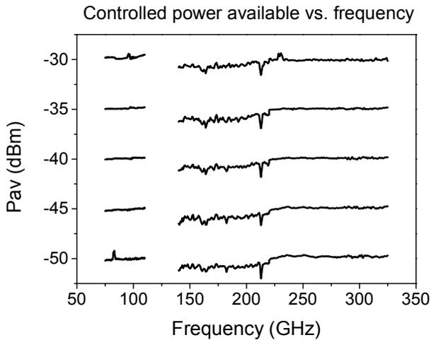
Fig. 4. Power available at Port1 of the proposed setup versus frequency in the WR-10, WR-5 and WR-3 waveguide bands, after power leveling. The plot shows the measured output power for different values of power set from the user, versus frequency.
