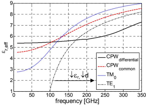
Fig. 2: Dispersion curves of the first propagating modes for the CPW (see Fig. 1) over alumina substrate with finite ground planes.
