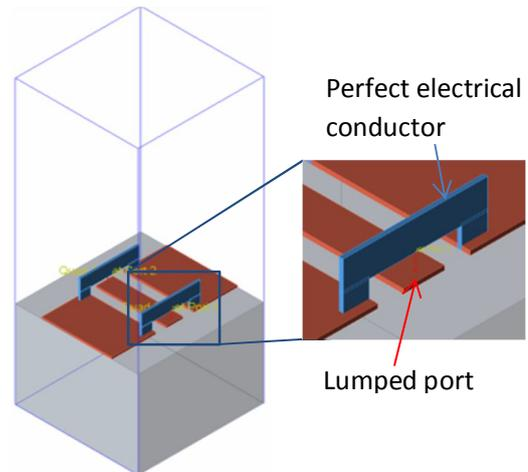
Fig. 6: 3D EM model of CPW and zoom-in of the lumped port used as stimulus, with boundary radiation box (blue box) directly set at the substrate edge (edge absorbing).
