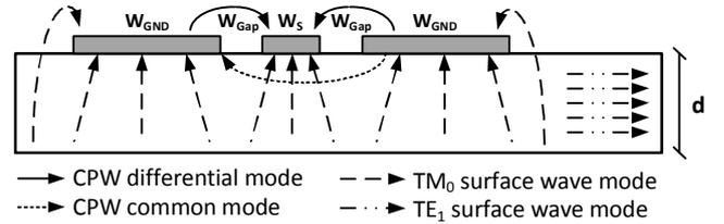
Fig. 1: Cross section of a CPW with finite ground planes, and sketches of the E field distributions of the first propagating modes supported.
