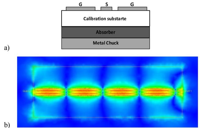
Fig. 4: a) Cross section of CPW on calibration substrate placed on the absorber interposer over the metal chuck, b) top view of the electrical field below the CPW, when using absorbing boundary below the substrate in the 3D FEM simulation, fields computed at 110GHz.
