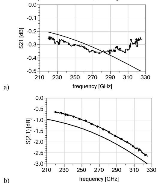
Fig. 12: Measured (line and symbols) and simulated data (solid line), after fused silica TRL calibration is performed. Measurement of structure from Table II, including metal and substrate loss (a), measurement of structure from Table I (b).
