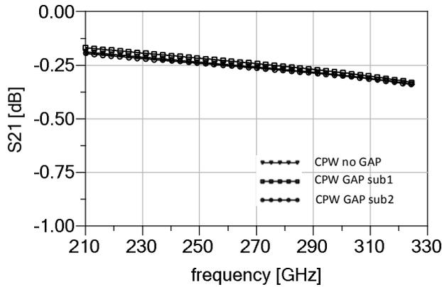
Fig. 10: Simulated S21 of CPW described in Table II for: case of structure shown in Fig. 6 (CPW no GAP), when substrate island is enlarged of 320  $\mu$ m and a gap of 500 $\mu$ m is applied between the substate and the absorbing box edge (CPW GAP sub1), and when substrate island is enlarged of 420  $\mu$ m and a gap of 500 $\mu$ m is applied between the substate and the absorbing box edge (CPW GAP sub2).
