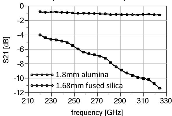
Fig. 14: Calibrated measured results of 1.8mm line on alumina and 1.68mm line on fused silica.
