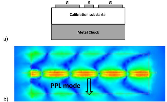
Fig. 3: a) Cross section of CPW on calibration substrate placed on metal chuck, b) top view of the electrical field below the grounded CPW metal plates, computed at 110GHz.
