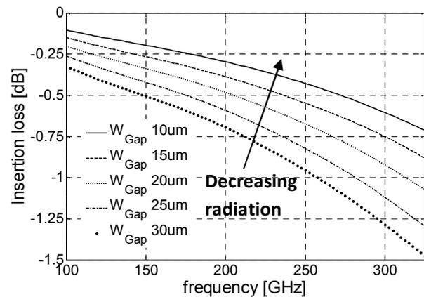
Fig. 5: Simulated insertion loss of CPW line described in Table I versus gap width, fixing the signal width to  $47.5\mu\text{m}$ . The CPW line is excited by a waveguide port.
