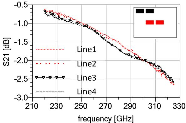
Fig. 13: Measurement of different (four) thru lines on alumina substrate in different location of the calibration substrate. Locations (i.e., two middle and two center) identified in the inset on top right.
