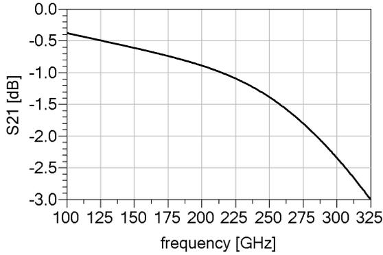
Fig. 7: Simulated S21 of CPW described in Table I when edge absorbing is considered (see Fig. 6).
