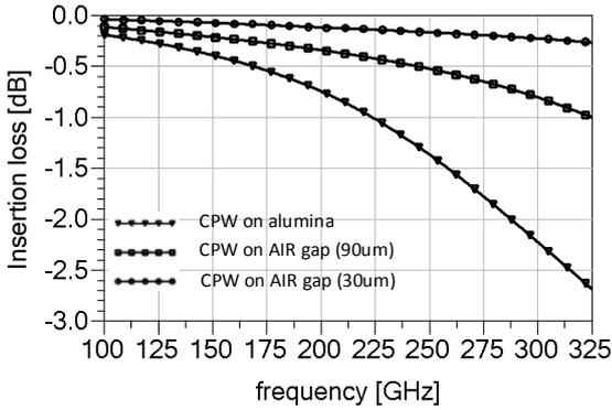
Fig. 8: Simulated insertion loss of the CPW structure described in Table I, compared to the air ( $\epsilon_r=1$ ) substrate case (CPW on AIR gap 30 $\mu\text{m}$ ) and the case with air substrate and an increased gap to account for the guided wavelength in the alumina (CPW on AIR gap 90 $\mu\text{m}$ ).
