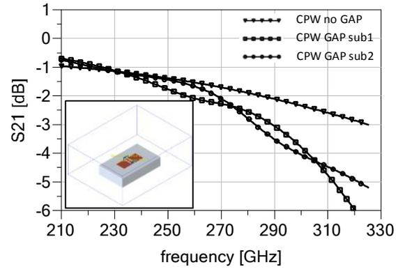
Fig. 9: Simulated S21 of CPW described in Table I for: case of structure shown in Fig. 6 (CPW no GAP), when the substrate island is enlarged of 320 $\mu\text{m}$  and a gap of 500 $\mu\text{m}$  is applied between the substrate and the absorbing box edge (CPW GAP sub1), and when substrate island is enlarged of 420 $\mu\text{m}$  and a gap of 500 $\mu\text{m}$  is applied between the substrate and the absorbing box edge (CPW GAP sub2).
