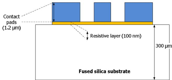
Fig. 1: Schematic cross section of the  $50 \Omega$  resistors fabricated on the proposed fused silica substrate
