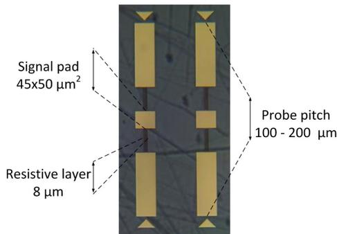
Fig. 2: Load standard artifact realized using the proposed technology
