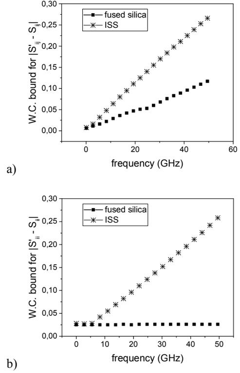
Fig. 4: Worst case error bound for a) measurements of transmission line and b) measurements of one port loads, obtained by using fused silica calibration (■) and ISS calibration (\*).
