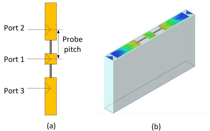
Fig. 3: a) Simulation setup in Keysight momentum for the load standard. The port positioning depends upon the targeted probe pitch. b) 3D model of the load standard after simulation, indicating field density over the conductor and resistive layer surface.
