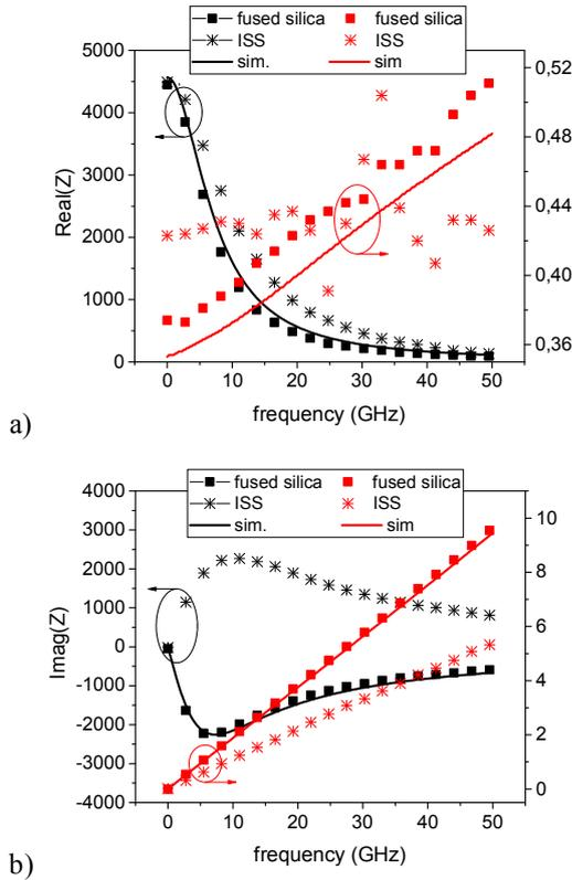
Fig. 5: a) Real and b) Imaginary part of the impedance extracted from the measurements of a 4500  $\Omega$  (black curves and symbols) and a 0.35  $\Omega$  (red curves and symbols) obtained by using fused silica calibration (■) and ISS calibration (\*) as compared to simulations (solid lines).
