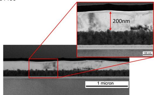
Fig. 12: TEM image of 200nm aluminum layer sputtered over a rough surface. As it can be seen by the inset the roughness is already absorbed after 200nm.
