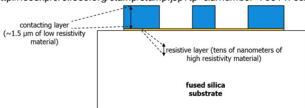
Fig. 10: Schematic cross-section of the 50 Ohm resistors fabricated on fused silica substrate.
