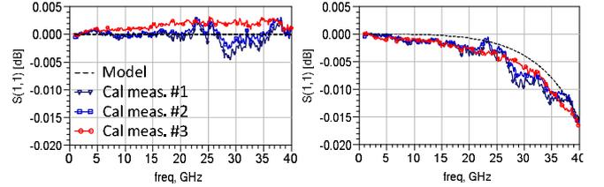
Fig. 3: Measurement versus model of the open standard: (left) employing standard model definitions, (right) employing EM extracted model definition for the calibration.
