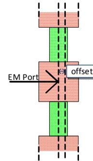
Fig. 6: Offset variable in parametric EM models used to propagate probe misplacement through different calibration algorithms.
