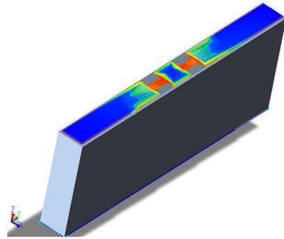
Fig. 1: 3D model of match load after Momentum simulation, indicating field intensity over the conductor and resistive layer surfaces.
