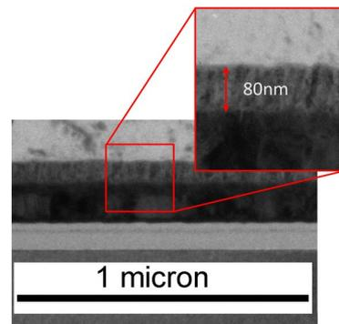
Fig. 13: TEM image of the resistive layer targeted to 80nm thickness.
