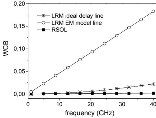
Fig. 8: Worst case error bound computed as in [10] from simulated data using as a  $450\mu\text{m}$  verification device line and employing the EM simulation of the line as the reference for the metric computation.
