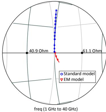
Fig. 2: Zoom-in of Smith chart presenting the standard model from the kit manufacturer and the EM extracted model for the load resistor.
