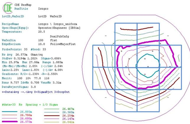
Fig. 11: Resistivity contour map over the 4 inch wafer, superimposed by the grid of  $2 \times 2 \text{ mm}^2$  dies. Measured standard deviation over 33 points over the entire wafer is 1.202%.
