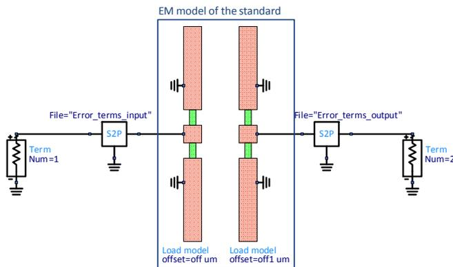
Fig. 5: Block diagram of measurement system, using experimental setup error model, implemented in Keysight's Advanced Design System (ADS) software.
