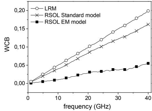
Fig. 9: Worst case error bound computed as in [10] from experimental data, using  $450\mu\text{m}$  line as a verification device and employing the EM simulation of the line as the reference for the metric computation.
