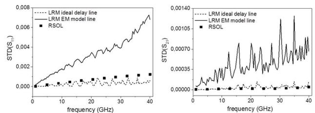
Fig. 7: Standard deviation computed from the Montecarlo simulation, for the magnitude of the reflection (left) and transmission (right) parameter for: the RSOL calibration (full squares), the LRM one employing an ideal delay line (dashed) or the realistic EM simulated line (solid).
