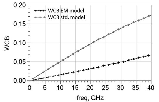
Fig. 4: Worst case error bound (WCB) as computed from equation 1, among three calibrated measurement employing the standard models ( $\circ$ ) and the EM derived models ( $+$ ).
